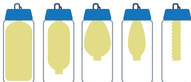
FIGURE 1. Depiction of an elastomeric pump as it delivers medication over time.
